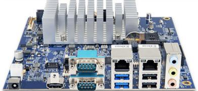
Fast-track the development of embedded systems for the most demanding industrial and commercial usage scenarios with the VIA EPIA-M930 Mini-ITX board. Combining a 1.8GHz Intel® Celeron® quad-core processor with a wealth of I/O and connectivity features, including support for up to three displays, the VIA EPIA-M930 provides a flexible and reliable platform for myriad applications based on a compact Mini-ITX form factor.
